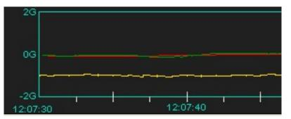
When then vehicle is static or "at rest" the lines will be nearly horizontal or charted in a straight line, with no deflection or charted deviation. Note the Z-axis charting is not at "0" as the vehicle is subject to gravity so there is a built in baseline at "1G" as long as the vehicle remains on planet Earth, caused by the forces of Earths gravity thus a permanent deflection baseline.
